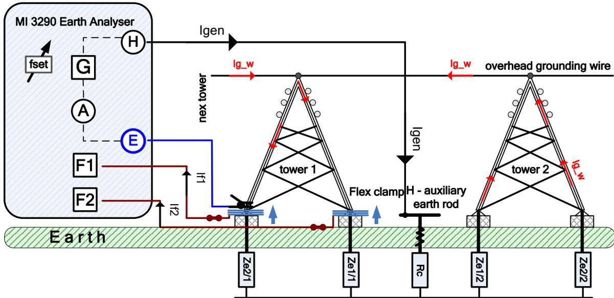
Figure 11.71: Pylon Ground Wire Test (PGWT) example
