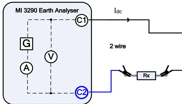
Figure 11.50: Ω - Meter (7 mA) example
