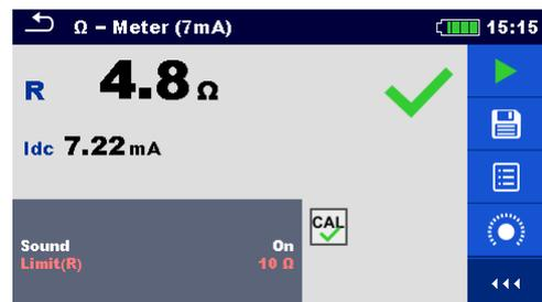
Figure 11.52: Example of Ω - Meter (7 mA) measurement result
