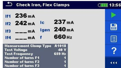
Figure 11.93: Example of Check Iron, Flex Clamps measurement result
