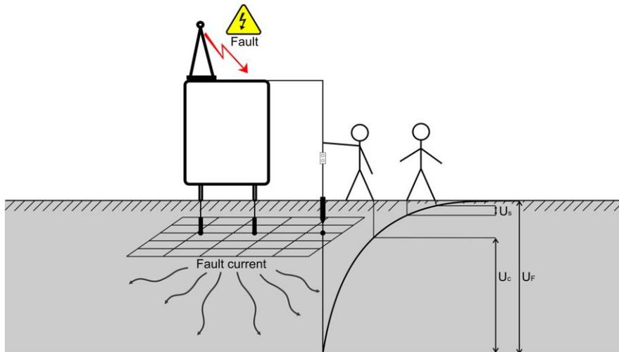
Figure 11.59: Dangerous voltages on a faulty earthing system
