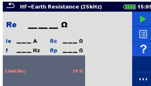
Figure 11.23: HF-Earth Resistance (25 kHz) measurement menu
