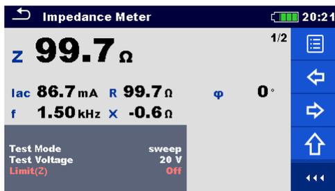
Figure 11.57: Example of Impedance Meter measurement result
