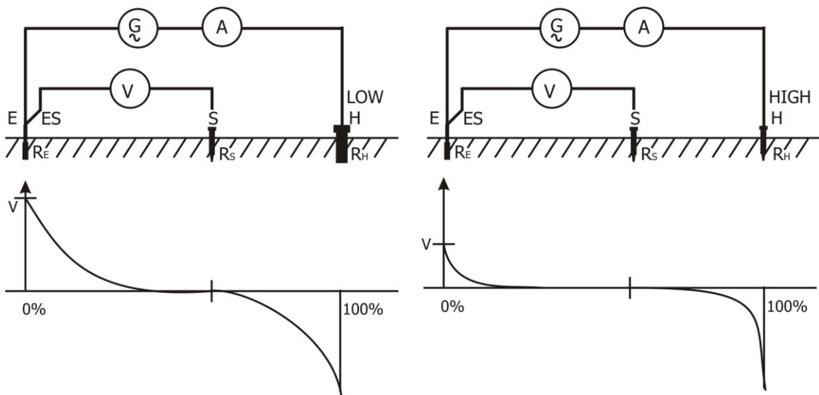
Figure C.6: Different measured voltage drops at low and high probe resistance
