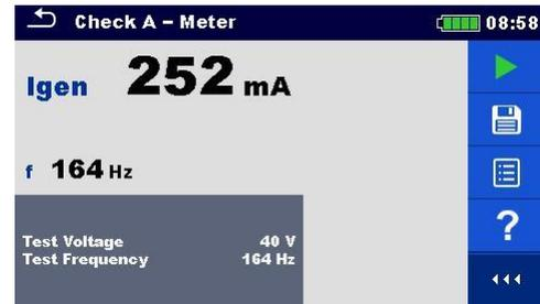
Figure 11.91: Example of Check A-Meter measurement result
