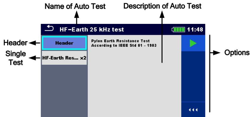
Figure 12.2: Auto test view menu – header selected
