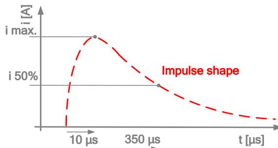
Figure 15.2: Typical Impulse shape short-circuit
