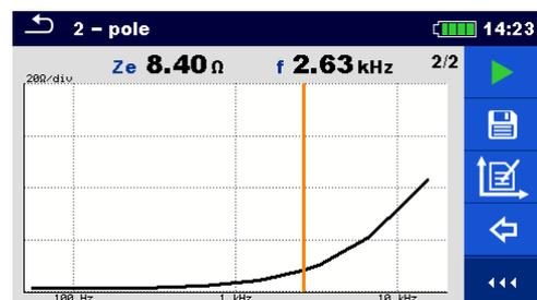
Figure 11.5: Example of 2-pole measurement graph view
