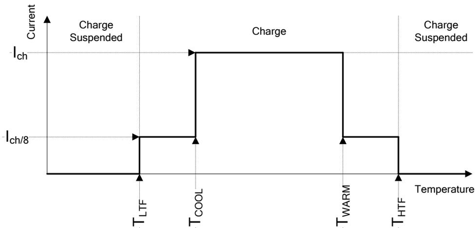
Figure 2.7: Typical charging current vs temperature profile
