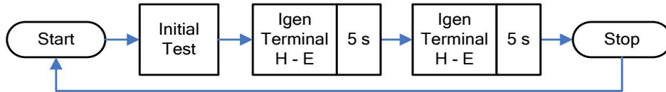
Figure 11.89: Check A-Meter measurement flow chart
