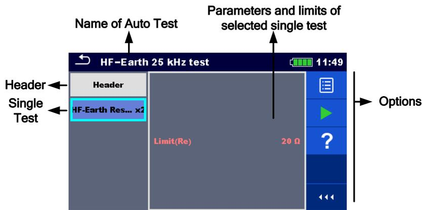
Figure 12.3: Auto test view menu – measurement selected
