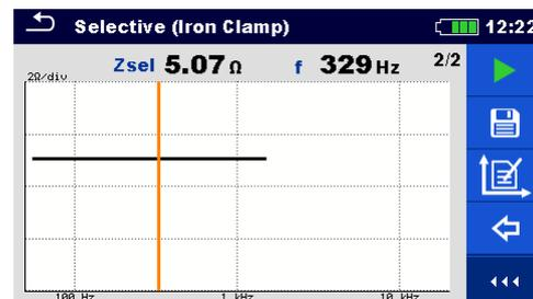
Figure 11.17: Example of Selective (Iron Clamp) measurement graph view
