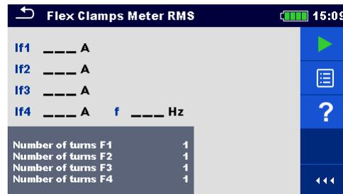
Figure 11.80: Flex Clamp Meter RMS measurement menu
