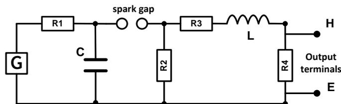
Figure 15.1: Simplified circuit of impulse generator in the MI 3290
