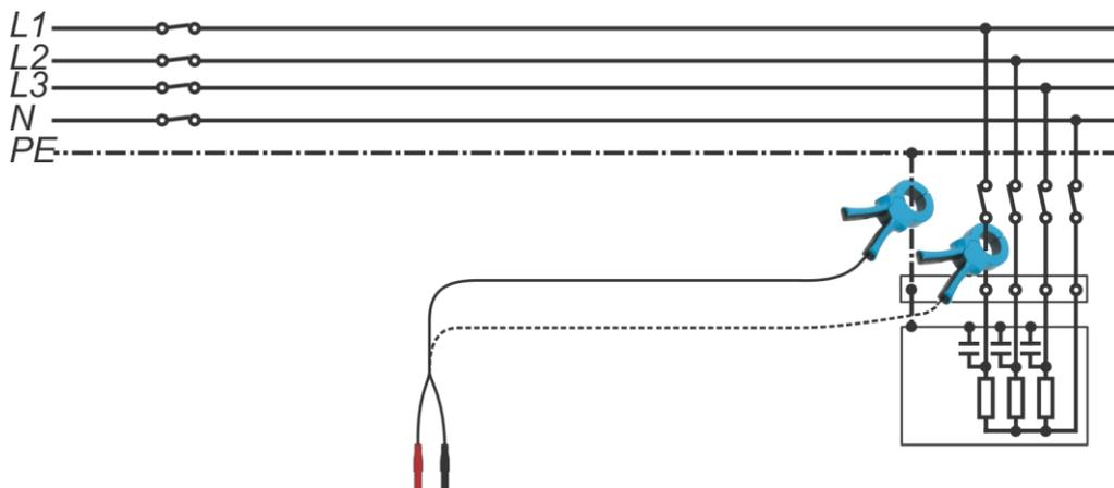
Figure 11.76: Iron Clamp Meter RMS example
