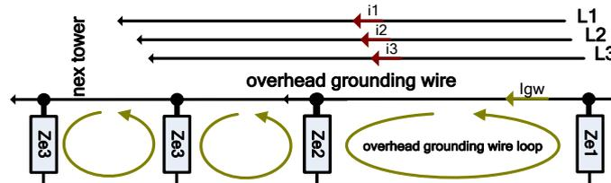
Figure 11.31: Substitute circuit for Passive (Flex Clamps) measurement
