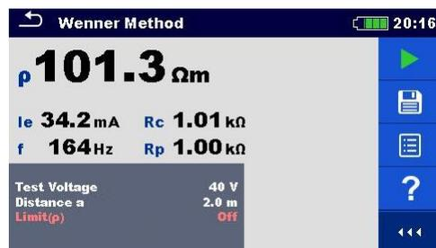
Figure 11.39: Example of Wenner method measurement result
