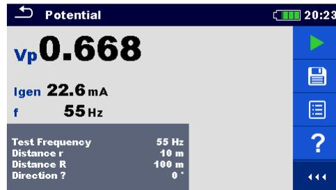
Figure 11.65: Example of potential ratio measurement result
