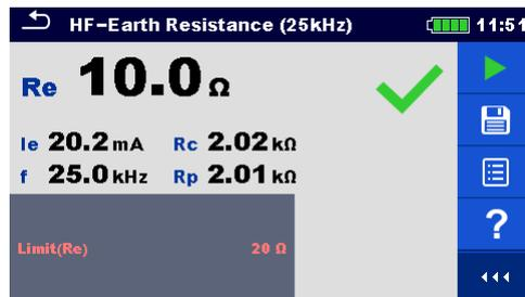
Figure 11.24: Example of HF-Earth Resistance (25 kHz) measurement result
