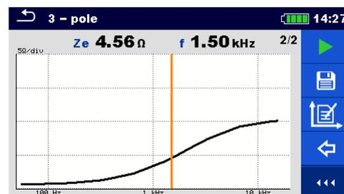
Figure 11.9: Example of 3-pole measurement graph view
