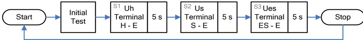
Figure 11.86: Check V-Meter measurement flow chart
