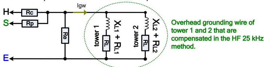
Figure 11.22: Compensation in HF 25 kHz method
