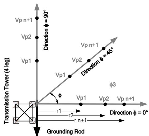
Figure 11.63: Potential gradient example (around the building)
