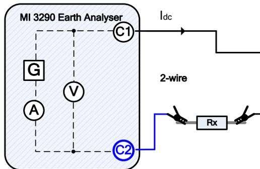
Figure 11.47: Ω - Meter (200 mA) example (2-wires)
