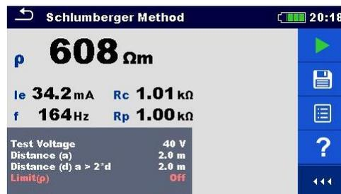
Figure 11.42: Example of Schlumberger method measurement result
