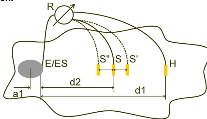
Figure C.3: Straight-line placement
