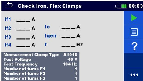
Figure 11.92: Check Iron, Flex Clamps measurement menu
