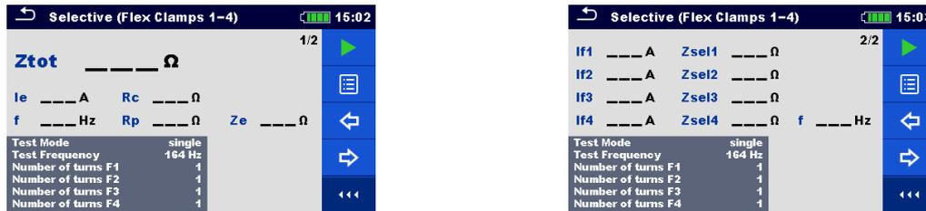
Figure 11.26: Selective (Flex Clamps 1-4) measurement menu
