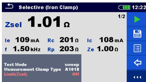
Figure 11.16: Example of Selective (Iron Clamp) measurement result
