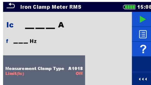
Figure 11.78: Iron Clamp Meter RMS measurement menu
