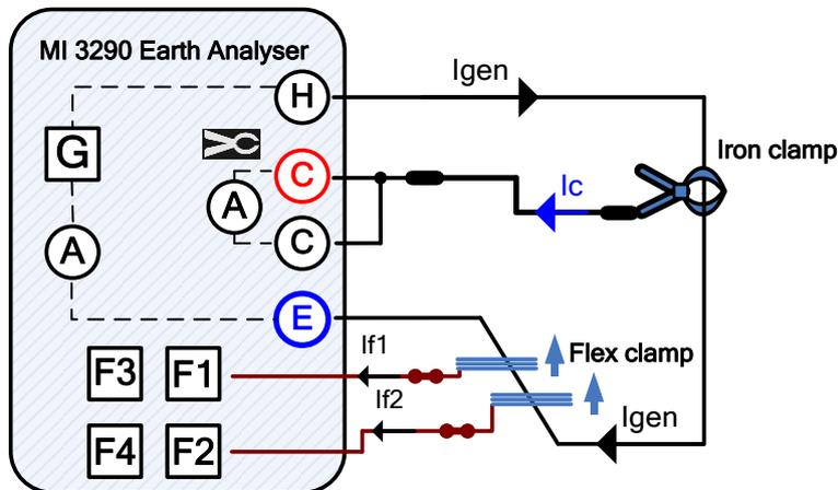
Figure 11.85: Checkbox measurements Iron, Flex Clamps example
