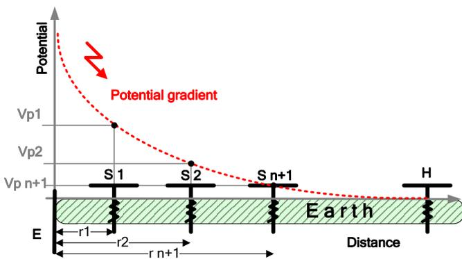
Figure 11.62: Potential gradient example (straight line)
