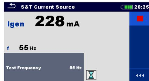
Figure 11.70: Example of S&T Current Source menu result
