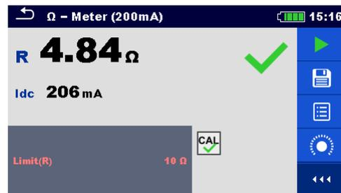
Figure 11.49: Example of Ω - Meter (200 mA) measurement result
