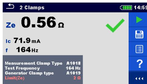
Figure 11.20: Example of 2 Clamps measurement result
